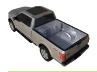
Developed and patented Nuchar® FuelSorb™ activated carbon monoliths that allow low-pressure (<1,000 psi) onboard natural gas fuel storage paired with conventional gasoline (bi-fuel hybrid).
